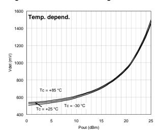
Figure 9. Power Detector Voltage Vs Pout
